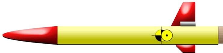
If the center of gravity and the center of pressure are in the same location, it is called **neutral stability**.
